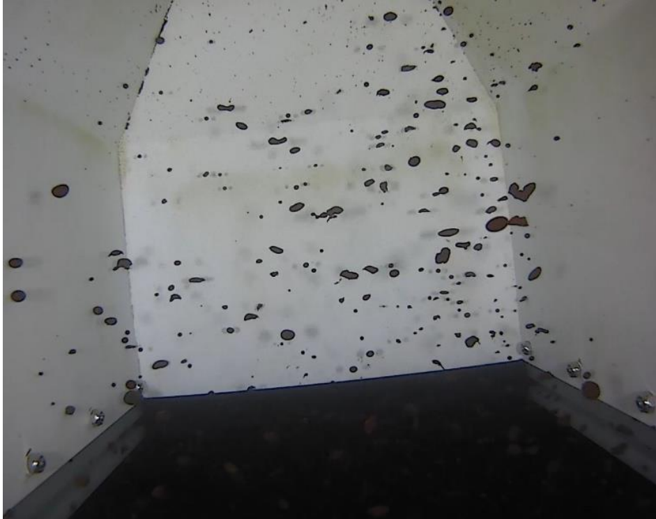
Exhibit 5: Screen shot from the NOAA/BSEE 2018 bubblemeter video showing the oil droplets being released from the oil-only plumes emanating from the pit near Dome C. For reference, the pan-head machine screws shown in this figure were 1/4" (6.35 mm), and have 7/16" (11.11 mm) lock nuts on the inside of the housing. A video clip is attached separately.
