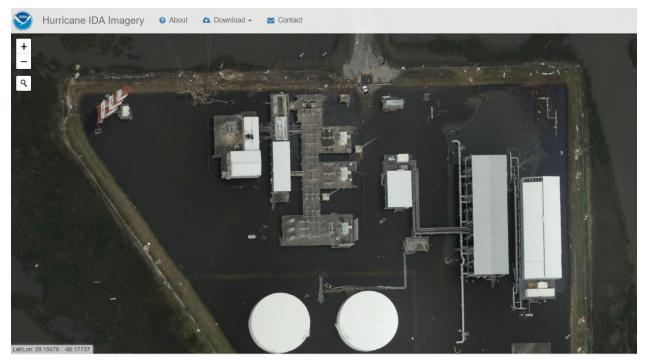
**Figure 9**. Hurricane Ida NOAA NGS Imagery of Shell Pipeline, Fourchon Booster Station, 31 August 2021. Oil sheen visible in the upper right corner of the enclosed facility in the image. <u>https://storms.ngs.noaa.gov/storms/ida/index.html#19/29.15662/-90.17502</u>
